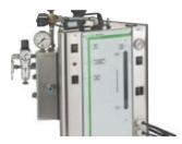
Larger steam generator also designed for producing steam to aid in curing junction liners. 22kg in weight, 9L boiler-refillable during operation, two heaters with 1500 watt for quick heating. Integrated pressure, vacuum and temperature control. Specifications: Max Power. 3KW / electric. Output approx. 4kg/hr - 100°C
